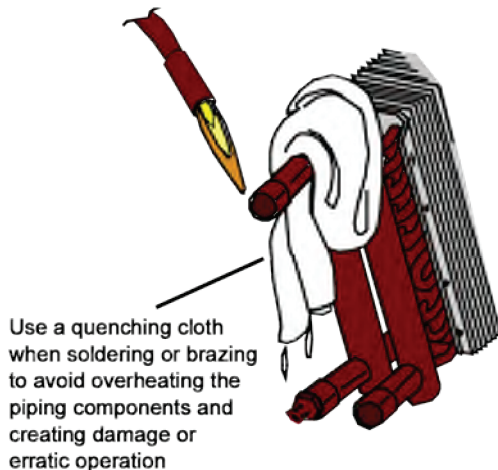
Figure 6: Protect Components from Overheating
